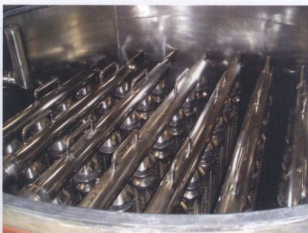
Internal view of Candle Filter
